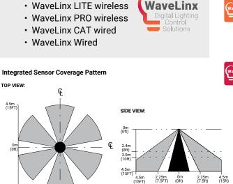
Note: Installation of integrated sensors within 3-ft (1m) of HVAC air vents is not recommended. The pattern shown is intended solely as a general guide and is not to scale.
