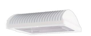
Specification Grade Area lights available in IES Type II distributions. For use in parking lots, roadways, pathways and general area lighting. Mounts to 4" square steel poles at 15-25'. Designed to replace 250W Metal Halide Area Lights. Patent Pending thermal management system. 5 Year Warranty.
