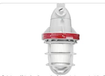
Explosionproof fixture for ceiling mounting. Set screw to stern prevents rotation. Cast aluminum housing, heat and impact resistant globe. Fits all incandescent lamps up to 300 Watt PS-25. Lamp not supplied.
